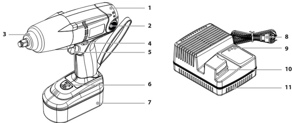
**1 Housing 2 Carbon brush 3 Shaft 4 Forward/Reverse handle 5 Switch trigger 6 Release button
