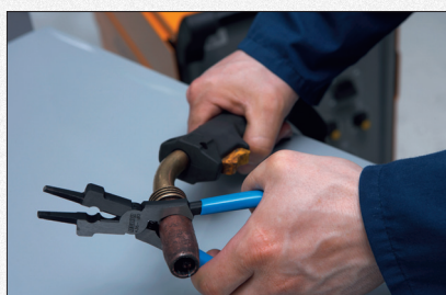
nozzle removal and installation
