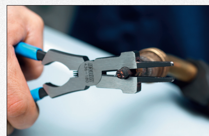
tip removal and installation
