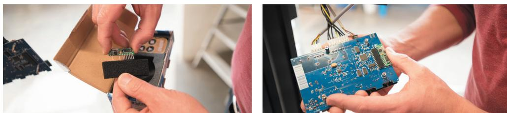
Install remote receiver into the socket connector on the bottom of controller. **Caution!** Remote receiver is electrostatic sensitive device. Avoid touching the contacts of Receiver before it is installed into the socket. Install receiver precisely to predefined location, marked with white rectangle on the controller.
