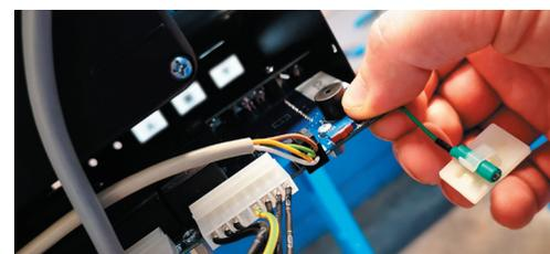
Install the controller back into the enclosure and fix it with four screws.
