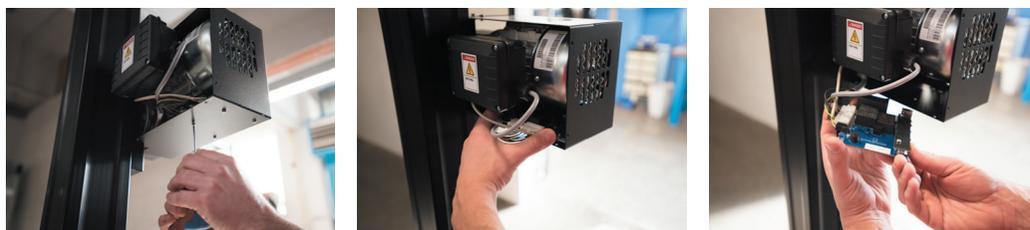
Unscrew and pull out the controller module - remove four screws at the bottom of enclosure (no need to disconnect cables from controller, it can be left out of enclosure by hanging on the cables).
