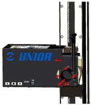
Unscrew top and bottom screws and disassembly motor protection and side protection from electric bike stand. Unscrew four screws from clamping head and remove it.
