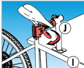
Firmly hold bike frame (I). Flip handle (J) to quickly release tube from jaws.
