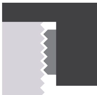
Sliding jaw with multiple positioning choices.
