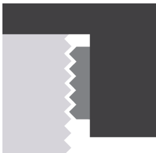
Sliding jaw with multiple positioning choices.
