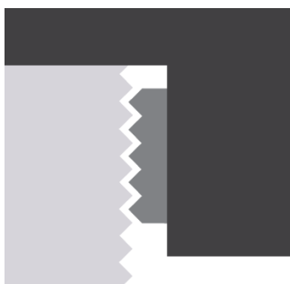
Sliding jaw with multiple positioning choices.
