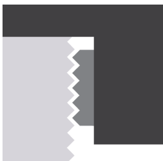
Sliding jaw with multiple positioning choices.
