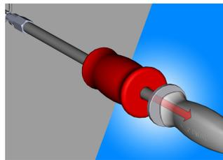
Start with steady hits extracting bearing with help of sliding hammer.
