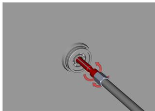
First inserted expandable collet through the hole in the bearing which will be extracted out of the housing. Then start to screw thorn into collet, which has a function that expands collet body, which adapts to the bearing bores.
