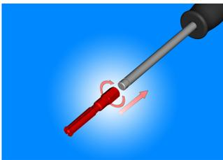
Before starting the application, you need to screw appropriate expandable collet dimension on the handle.
