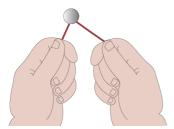
Thread the safety wire through your fastener(s) in the appropriate manner. You will now have two ends of the wire ready to twist.
