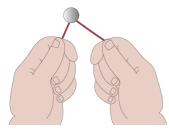
Thread the safety wire through your fastener(s) in the appropriate manner. You will now have two ends of the wire ready to twist.
