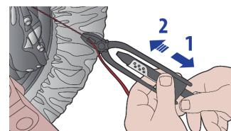
Let go of the plier handles and pull the chrome handle at the base of the pliers to rotate the pliers and twist the wire in a clockwise direction.
