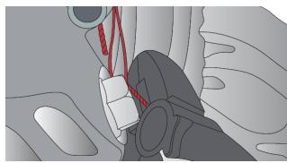
Squeeze the plier handles to release the chromed locking slider, and then use the integrated wire cutter to trim the wires to length.
