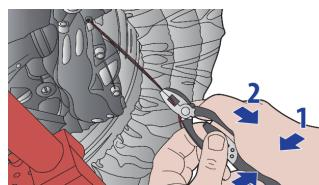
Slide the central chromed locking sleeve to lock the plier handles together, clamping the wire ends.
