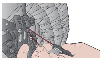
Use the safety wire twisting pliers to grip the two wires at an appropriate distance from the fastener. The length of wires between the pliers and the fastener will be twisted in the following step.
