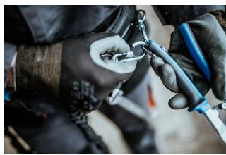
The carabiner on the lanyard is attached to the ring on the tool. The rings on the tools are large enough to accept 2 carabiners.
