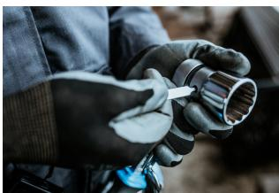
Using the socket remover (Article 1111) depress the pin in the hole while removing the socket from the square drive of the ratchet and then switch the socket or extension.
