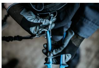
Before removing the tool from the belt, unscrew the lock ring on the carabiner on the belt.
