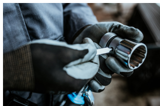
Using the socket remover (Article 1111) depress the pin in the hole while removing the socket from the square drive of the ratchet and then switch the socket or extension.
