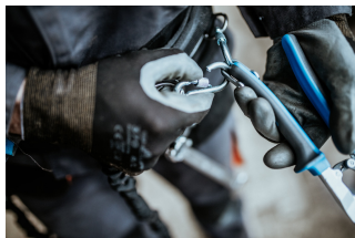
The carabiner on the lanyard is attached to the ring on the tool. The rings on the tools are large enough to accept 2 carabiners.
