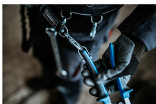
Correct attachment of the tool to the lanyard. Return the tool to the belt following the steps in reverse order.
