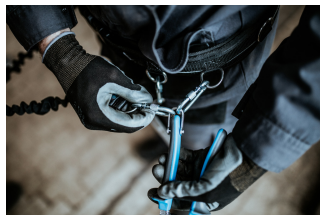
The carabiner on the lanyard has to be protected against opening using a lock ring.
