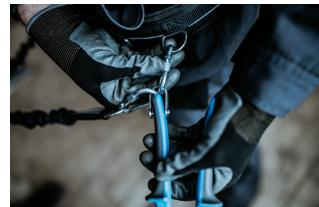
Before removing the tool from the belt, unscrew the lock ring on the carabiner on the belt.
