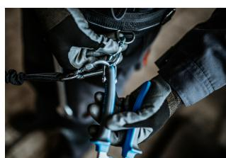
Open the carabiner on the belt and remove the tool, which is attached to a lanyard, from the carabiner on the belt. The tool is now ready for use.
