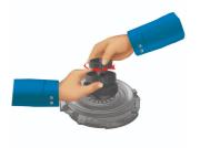
Keeping the knob (2) in place, turn knob (1) and block the expanding cone in the centre of the clutch disc.
