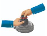
Keeping the knob (2) in place, turn knob (1) and block the expanding cone in the centre of the clutch disc.
