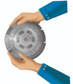
Manually centre the disc on the spring plate.
