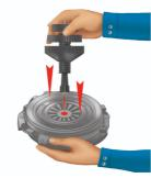
Turn the knob (3) until it touches the knob (2). Keeping the regulating screw still, unscrew the knob (1) and support it against the knob (2). Insert the device in the centre of the gear disc, passing it through the spring plate and press down.
