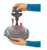
Turn the knob (3) until it touches the knob (2). Keeping the regulating screw still, unscrew the knob (1) and support it against the knob (2). Insert the device in the centre of the gear disc, passing it through the spring plate and press down.
