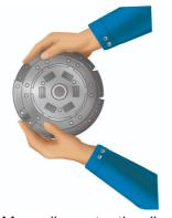
Manually centre the disc on the spring plate.
