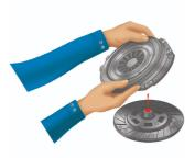
Place the spring plate on the clutch disc.
