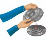
Place the spring plate on the clutch disc.
