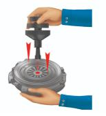
Turn the knob (3) until it touches the knob (2). Keeping the regulating screw still, unscrew the knob (1) and support it against the knob (2). Insert the device in the centre of the gear disc, passing it through the spring plate and press down.
