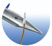
The pliers can be used for crimping insulated spade terminals.
