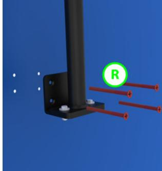
Mount stand on wall? To mount the stand to the wall, prepare the holes with drill size 10 mm and use attached screw anchors and screws (R).
