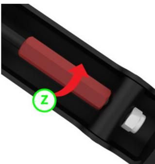
To adjust jaw opening, turn the long screw (Z) with hand in needed direction.
