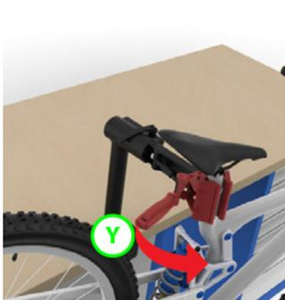
Release bike from stand? To release, firmly hold bike frame. Flip handle (Y) to quickly release tube from the jaw.
