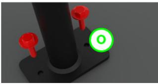
Mount stand on wooden bench? To mount the stand on a wooden bench, prepare the holes with drill size 6 mm and use the attached screws (O) as shown on picture.
