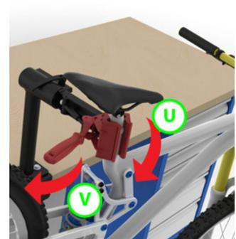
Adjust opened jaw (U) to seatpost or bike tube. Turn handle (V) until jaw firmly grabs the tube.
