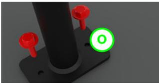
Mount stand on wooden bench? To mount the stand on a wooden bench, prepare the holes with drill size 6 mm and use the attached screws (O) as shown on picture.
