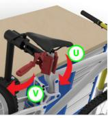
Adjust opened jaw (U) to seatpost or bike tube. Turn handle (V) until jaw firmly grabs the tube.
