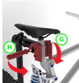
Adjust opened jaw (G) to the seatpost or bike tube. Turn handle (H) until jaw firmly grabs the tube.
