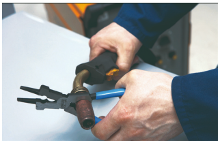
Nozzle removal and installation
