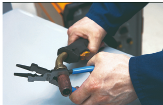
Nozzle removal and installation
