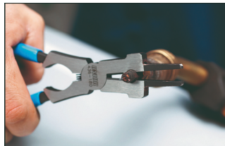
Tip removal and installation
