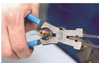
Installation bushing removal and installation
