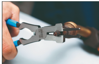
Tip removal and installation
