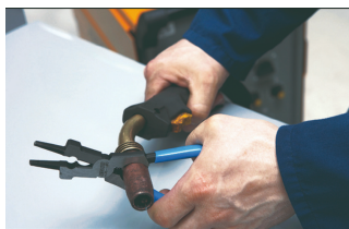
Nozzle removal and installation
