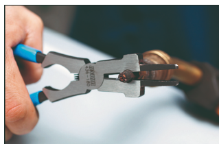
Tip removal and installation
