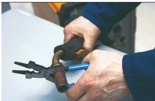
Nozzle removal and installation
