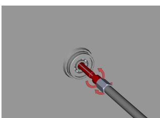
First inserted expandable collet through the hole in the bearing which will be extracted out of the housing. Then start to screwed thorn into collet, which has a function that expands collet body, which adapts to the bearing bores.
