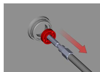
After several strokes fast and easy extract bearing from housing without damage.
