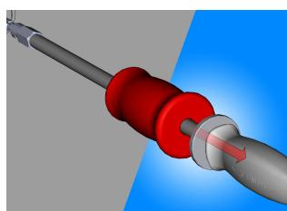
Start with steady hits extracting bearing with help of sliding hammer.
