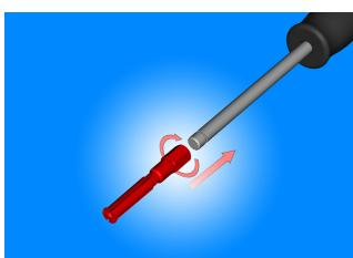
Before starting the application, you need to screw appropriate expandable collet dimension on the handle.
