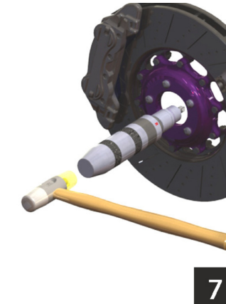
When the tool is properly positioned on the screw, tap the tool holder with hammer. This will trigger mechanism that allows bolt tightening/loosening for approx. 15°.
