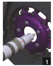
Move impact screwdriver closer to screw, which we will tighten (R), or loosen (L)
