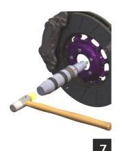
When the tool is properly positioned on the screw, tapp the tool holder with hammer.
