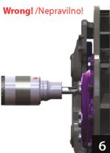
When the tool is in the compressed position, and we strike it with hammer inner mechanism will get destroyed. Never strike tool with hammer, when the tool is in compressed position!
