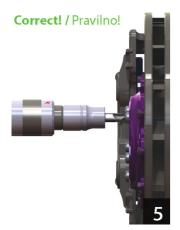
Move tool closer to screw, and dont press it to final position before use. With hammer strike, tool is automaticlly extracted and tightening/loosening begins.
