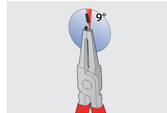
The tips are inserted into the jaw at an angle that prevents the circlip from sliding off the tips
