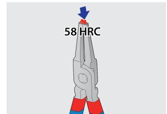
Tips hardened to 58 HRC prevent bending or breaking during the removal or insertion of circlips
