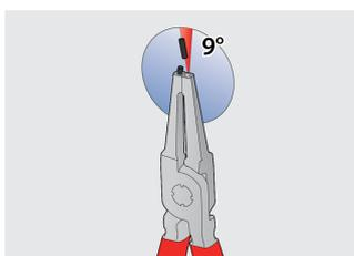
The tips are inserted into the jaw at an angle that prevents the circlip from sliding off the tips
