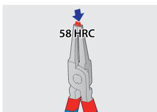
Tips hardened to 58 HRC prevent bending or breaking during the removal or insertion of circlips
