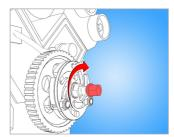
Turn spindle clockwise until pulley comes off.
