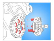
Insert puller legs into openings of pulley.
