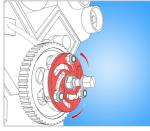
Turn setting plate to shift puller legs, so they tightly grasp to pulley.
