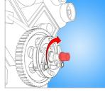
Turn spindle clockwise until pulley comes off.
