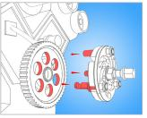
Insert puller legs into openings of pulley.
