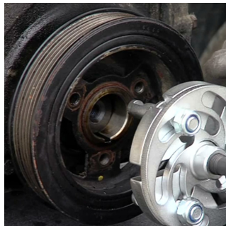
Turn setting plate to shift puller legs, so they tightly grasp to pulley.
