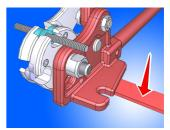
Important notes when cutting; When operating on the floor, apply foot pressure on the bracket.
