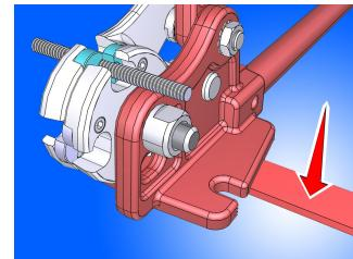
Opening the cutter; To operate correctly, the cutter should be opened by raising the top lever handle to its maximum extent. When fully open, insert the threaded rod into the cutter opening of the corresponding dimension.
