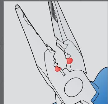
Stripping off insulations from  $\varnothing$  3.5 mm to  $\varnothing$  4.0 mm.
