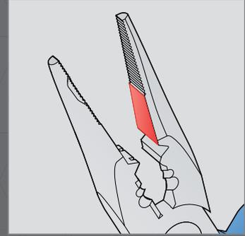
The ground part of the jaw is intended for gripping objects with sensitive surfaces.
