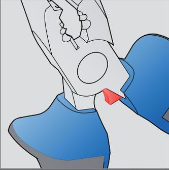
Crimping cable terminals up to  $\varnothing$  4.0 mm.
